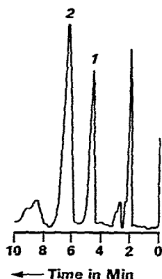
Fig. 1. Chromatogram of patient sample. Solvent, 1% propionic acid-methanol (80:20) adjusted to pH 5.0 as described in the text; flow-rate, 1.7 ml/min. 1 = Theophylline, 2 = 8-chlorotheophylline.
